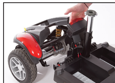
Step 4: Pull forward on the drivetrain release lever to separate the front and rear frame sections!
