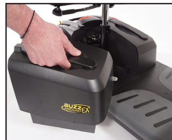
Step 2: Pull out the battery pack!
